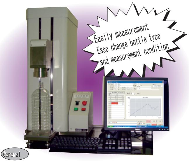
This equipment is measuring the maximum load and displacement of body bending and displaying the real-time data on computer display and total up the data. It is possible to measure automatically with robot I/O signal (Option at order)
